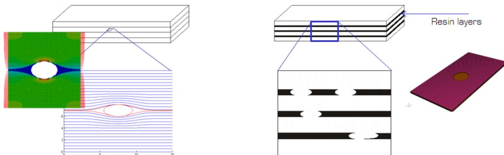
Figure 1: Unidirectional layer with void inclusion under compressive loading.
