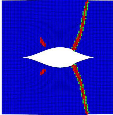
Figure 2: Progressive failure under compression load, colors indicate the damage state
